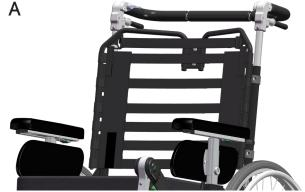
The Flexi-back system provides an adaptable support and is suited to backs without deformities as well as those with, for example, thoracic kyphosis. It consists of a Flexi-frame with straps, 7 for Standard and 8 for Long. The straps make it possible to regulate the pelvic position, provide support for the lower back, and thus achieve a more upright sitting position. The back cushion is attached to the backrest with velcro (B).
